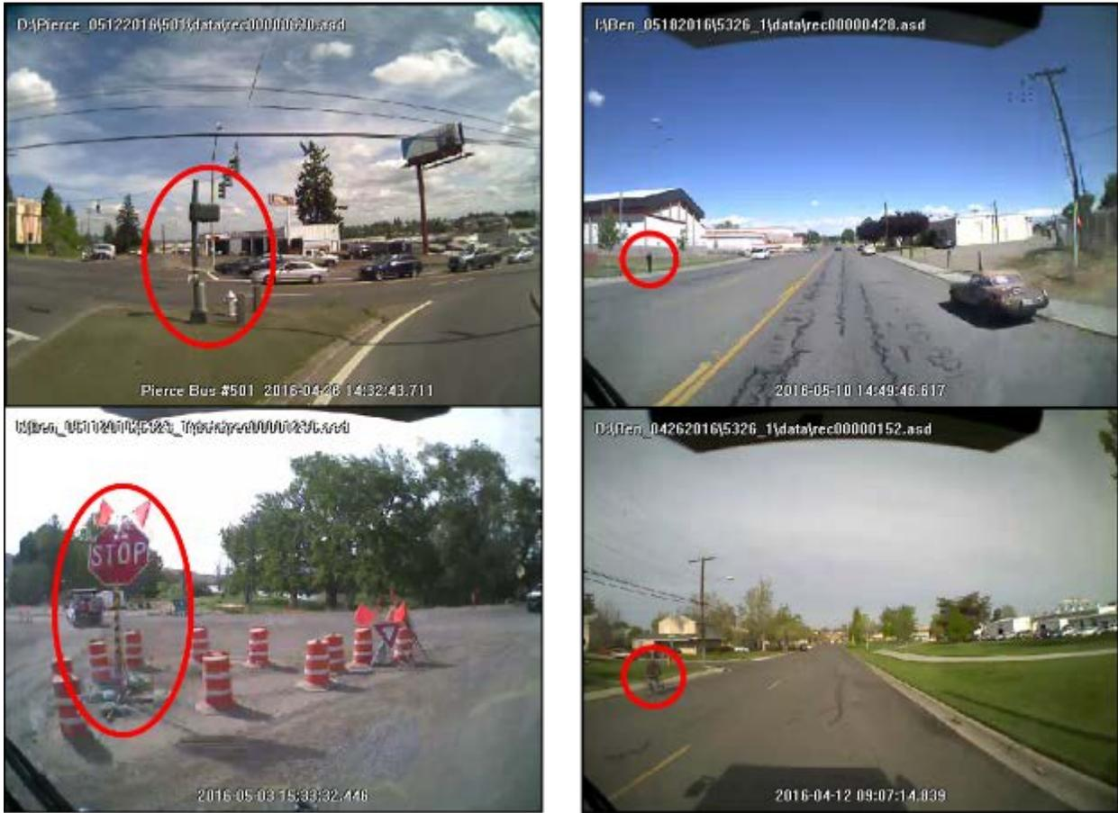
**FIGURE 9 Examples of Late Detections Identified as False Negatives**
