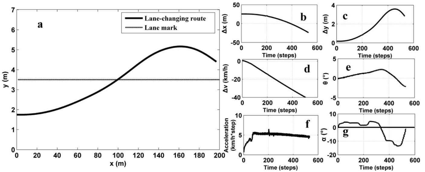
Fig. 4. Example of lane-changing route and data samples collected in the scenario with speed of 60 km/h.
