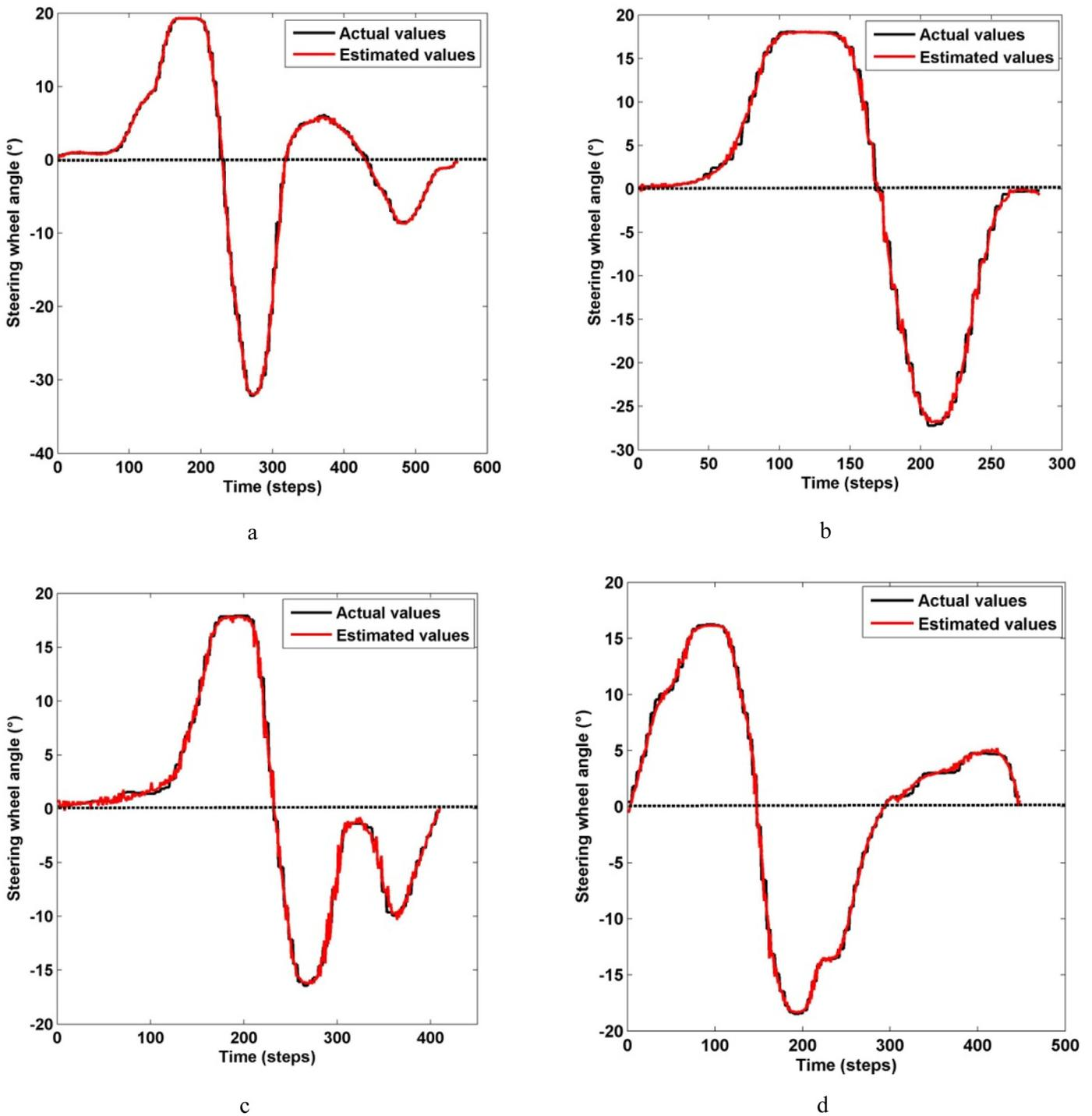
Fig. 9. Prediction results of steering angles for four drivers in scenario with speed of 80 km/h.
