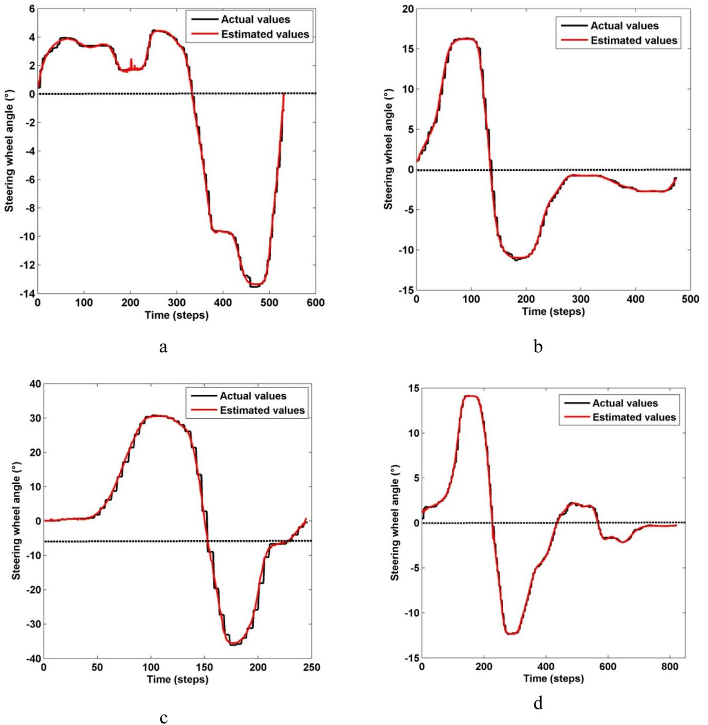
Fig. 8. Prediction results of steering angles for four drivers in scenario with speed of 60 km/h.
