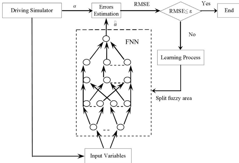
Fig. 2. Structure of prediction system.
