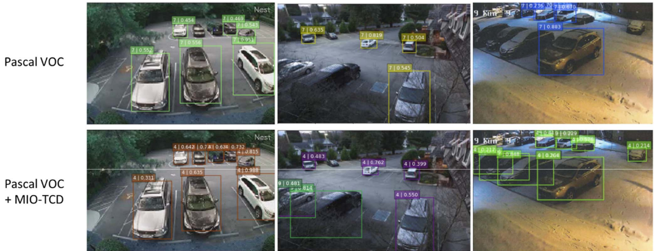
Fig. 3. The enhanced SSD-Mobilenet Detector implemented at the edge of our system has a significantly improved detection performance, especially on challenging parking scenarios in surveillance image data.
