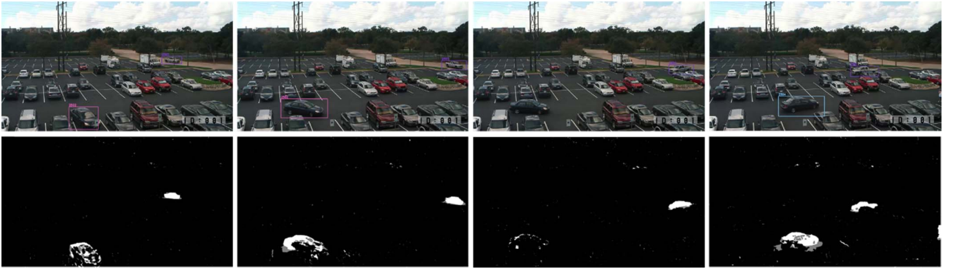
Fig. 4. BG-based detection and the original SORT tracking results. In a parking lot scene, the car at the bottom-left is lost with an ID switch due to its stop to change direction. Our modified SORT algorithm on the server solves this problem, thus reduce the error in parking occupancy detection.
